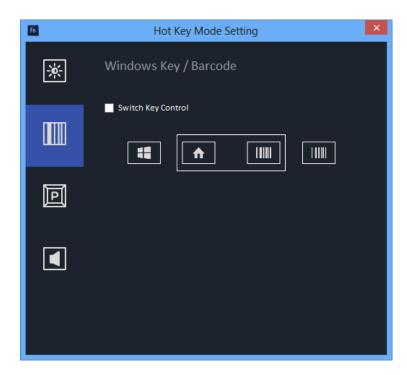
Once the hot keys are set to Windows Home & Barcode Trigger mode, the barcode will be turned on automatically. Users can press barcode trigger hot key to scan any barcode and the barcode information can show in the notepad or word file.
