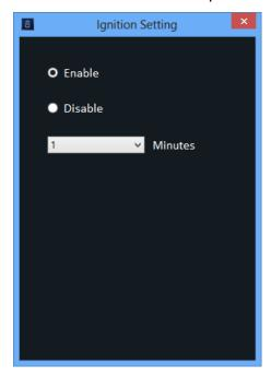
When PWS-872 is docked and vehicle is turned to ignition off, the PWS-872 will pop up a countdown warning message as below. User can tap OK to turn off PWS-872 or tap Cancel to keep PWS-872 on. If not action is taken, PWS-872 will automatically shut down after countdown period.
